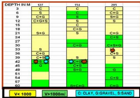
Fig. 2 Near-surface velocity and lithology in the vicinity of analyzed shots ( from up-hole survey)
