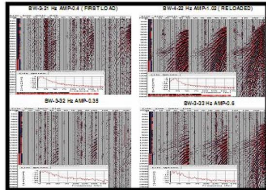
Fig. 3 Field monitor records (raw) of first time blasted (left) and re-blasted (right) in sand layer
