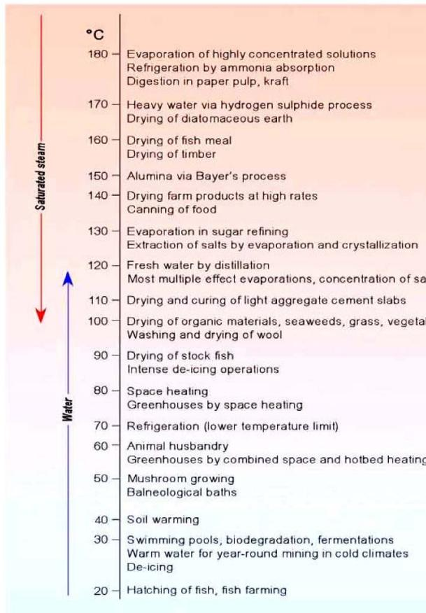
Figure 1: Lindal Diagram: Temperature requirements of geothermal fluids for various applications
