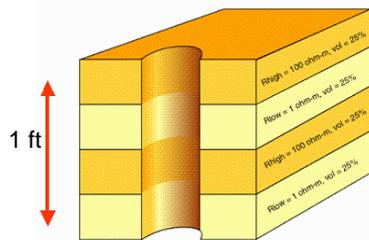
When thin laminae of sand and shale are intersected by a wellbore, electrical current from the resistivity tool is shorted due to the high conductivity of the shale laminae. Consequently, the hydrocarbon-bearing sand layers, although being more resistive may not be detected. When producing thin-bedded reservoirs, the contributions of many laminae will be cumulated together.
