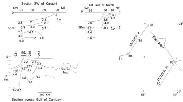
Figure 4: Refraction seismic sections of Western Offshore, India
