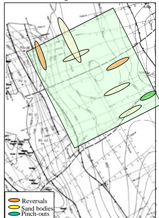
Fig.2 Time structure map on top of Mid. Bhuban, Agartala Syncline
