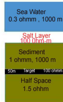
Figure 3.1D model of hydrocarbon reservoir below the salt layer.
