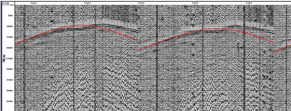
Figure 5: Field Raw Record shown in figure 4 with LMO (in red) picked with lower velocities confirming the geometry on the left part of the split spread.
