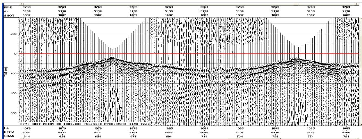
Figure 2: Field Record shown in Figure: 1 with flattened LMO (picked from other shots in red colour). The first breaks near the shot show a hump giving the impression of geometry error.
