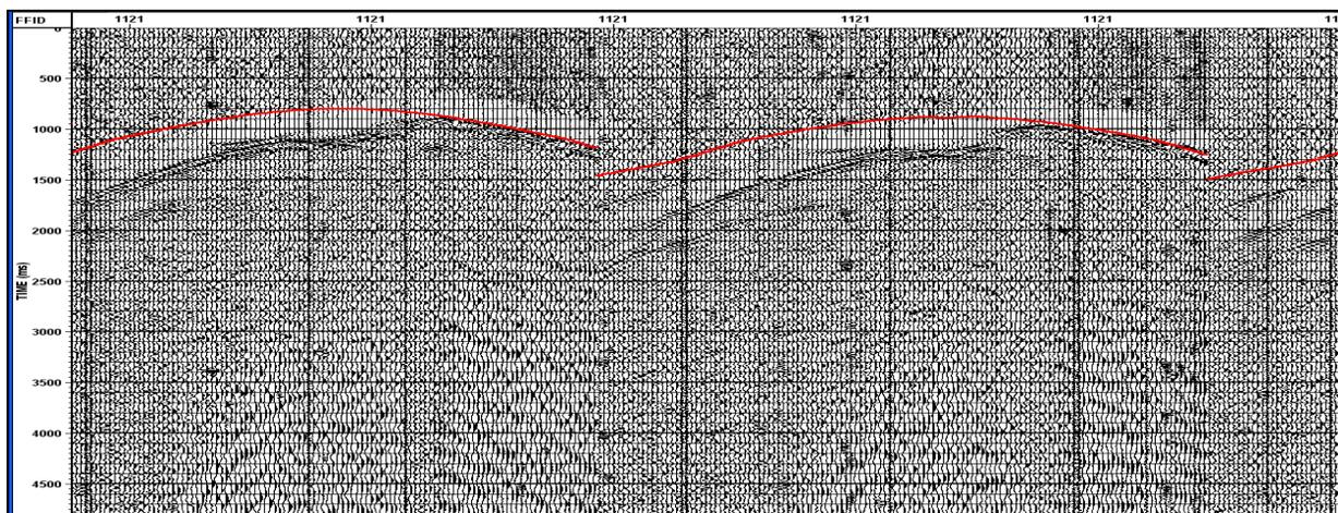
Figure 6: Field Raw Record shown in figure 4 with LMO (in red) picked with higher velocities confirming the geometry on the right part of the split spread.
