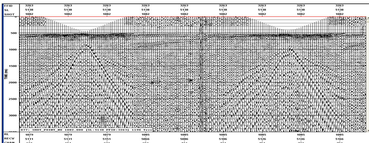
Figure 3: Field Record shown in figure 1 with flattened LMO (repicked velocity in red colour). The first breaks are parallel to the LMO confirming the geometry.
