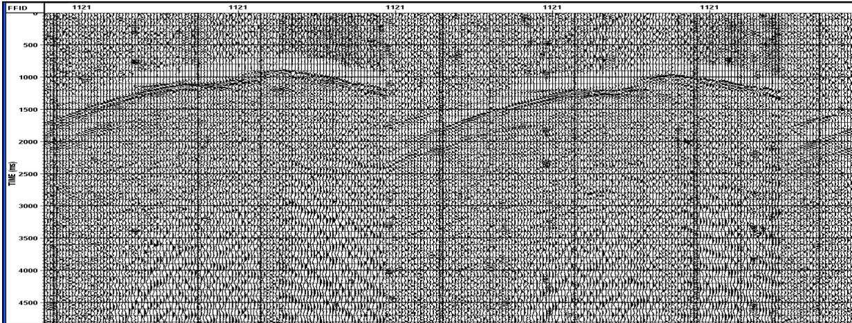
Figure 4: Field Raw Record from a geologically complex area with one part of the split spread over exposure of older beds and the other part of the spread on alluvium covered area.
