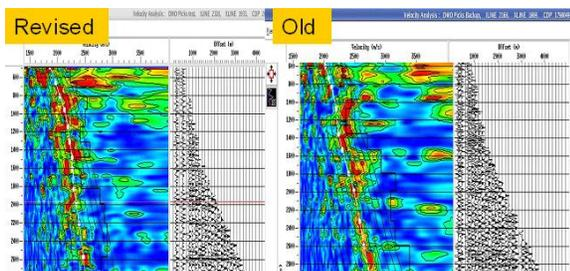
Fig: 2 Missing picking links at shallow levels due to multiple signal responses are taken care of in the refinement. (a) Revised velocity panel , b) old velocity panel.
