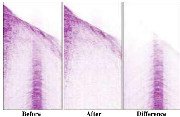
Figure 7: Example for Rig noise elimination test.
