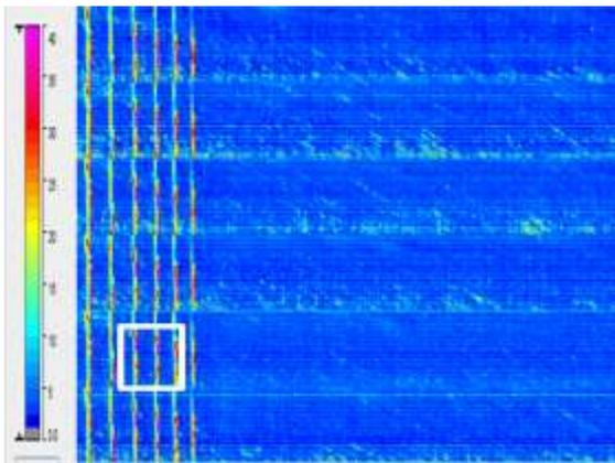
Figure 2: Seismic Interference (red, >25  $\mu$ Bar RMS, move out 310 ms/km), all 6 streamers on background RMS amplitude plot.
