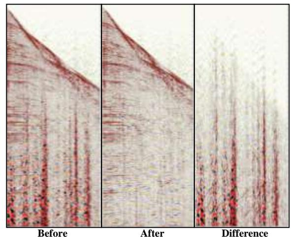
Figure 11: Example of swell noise attenuation test, performed in the white box region of figure 7.
