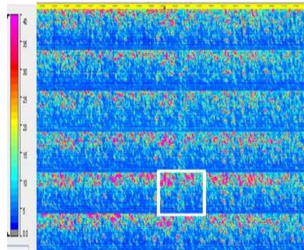
Figure 10: Effect of swell noise (red, >25  $\mu$ Bar RMS) for all 6 streamers on background RMS plot.
