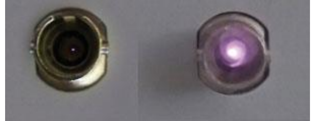
Figure 4 Infra-red signal seen through a mobile phone camera
