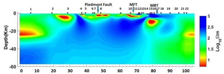
Figure 3: Profile section extracted from 3D model obtained from full impedance inversion with 100  $\Omega\text{m}$  half-space as initial guess.
