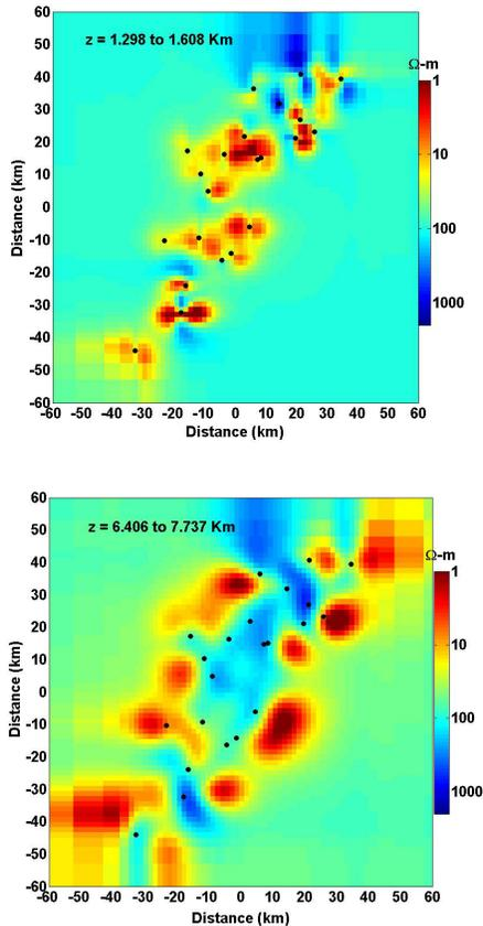
Figure 4: Depth plane slices of 3D inverted model full impedance. The depth at which these planes are extracted are 1.29 to 1.609 KM; 6.4 KM to 7.37 KM.
