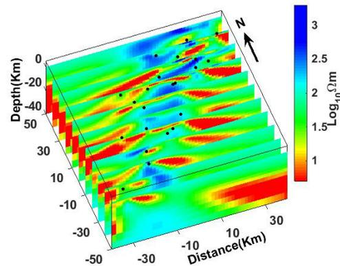
Figure 2: 3D model YZ plane slice of the inverted model obtained after inversion of (a) full impedance data with 100 ohm-m half-space as initial guess.
