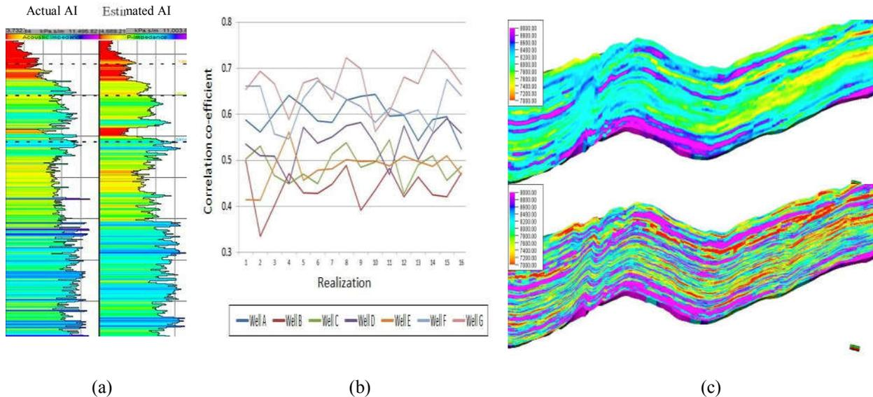
Figure 4 Stochastic Inversion results (a) Blind well test at Well A. 4(b) Blind well test correlation matrix run for 7 wells and 16 realizations. 4(c) Comparison between the resolution of deterministic AI(top) and stochastic AI(bottom) for one section. Red, yellow and green colors are highlighting the sand packages.
