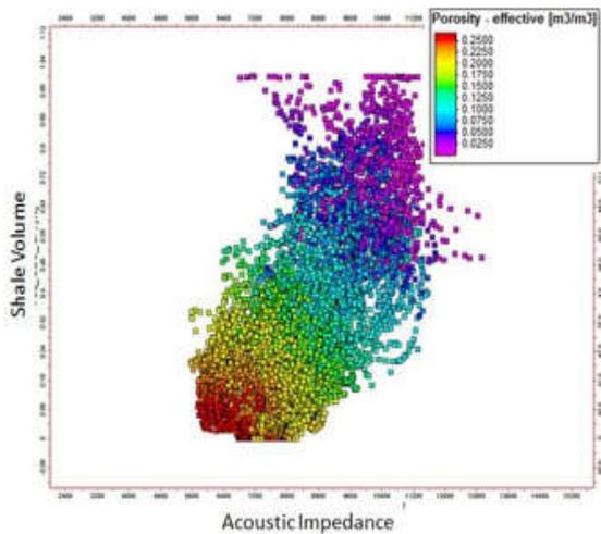
Figure 5 Rock Physics Analysis - Vshale vs Acoustic Impedance plot for Zone 2, colored by Effective Porosity values, showing a good relation between the well logs.
