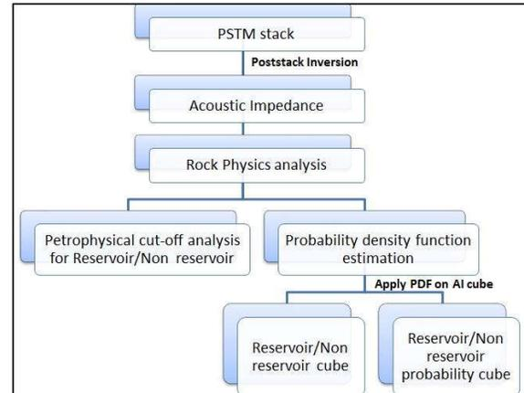
Figure 2: The workflow followed to build a litho-cube in this study.
