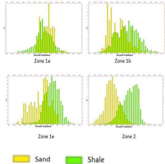
Figure 6 Rock Physics Analysis - Acoustic Impedance histograms for 4 zones, showing the sand shale delineation in some of them.
