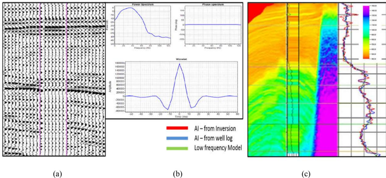
Figure 3(a) Seismic well tie of Well A. 3(b) Wavelet extracted from Well A. 3(c) Simultaneous Inversion match at Well A.
