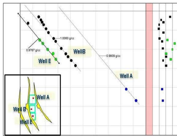
Figure 1a. (inset) Fault interpretation indicates Well A, Well B and Well E are drilled in same fault block, hence should be in hydro dynamic equilibrium.
