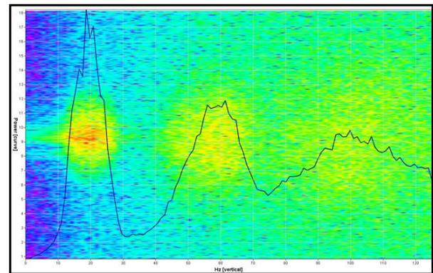
Figure 4(b): Frequency spectrum of data after cosmetic enhancement showing a bandwidth extension with the high frequency component
