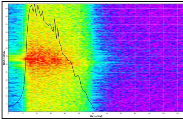
Figure 2(d): Frequency spectrum of original 3D PSTM seismic data
