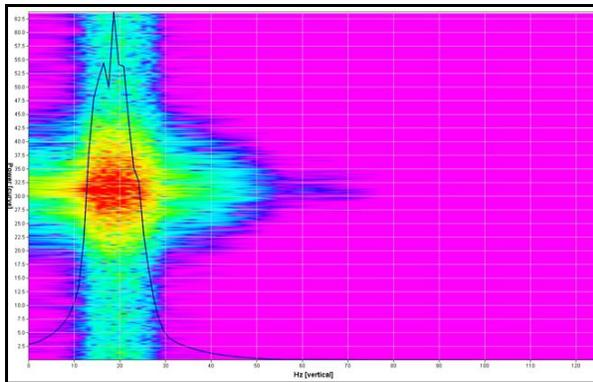
Figure 3(b): Frequency spectrum of the graphic-equalized seismic volume showing dominance of frequencies in between 10-30 Hz
