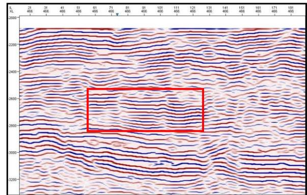
Figure 4(a): Cosmetic enhancement of median filtered seismic data showing an increase in the sharpness of the events and also pinch-outs and truncations of events
