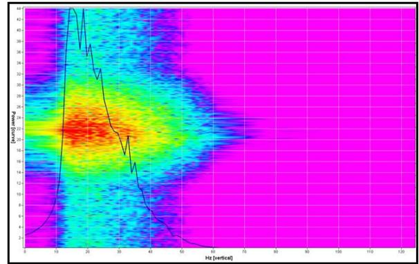
Figure 2(e): Frequency spectrum of median-filtered 3D PSTM seismic data showing an attenuation of high frequency component from the original seismic data
