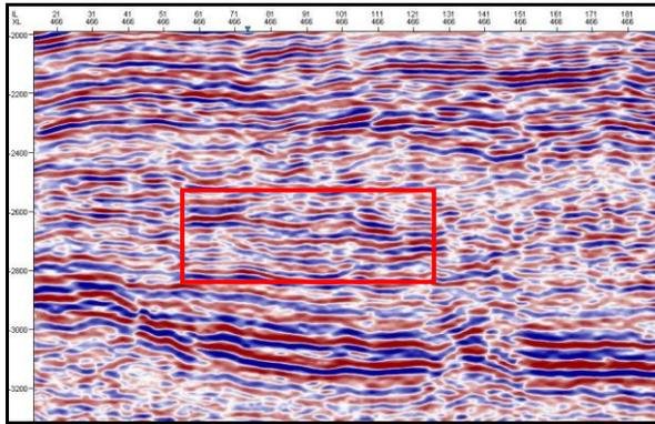
Figure 2(b): Median filter with filter width of 3X3 applied on original 3D PSTM seismic data.
