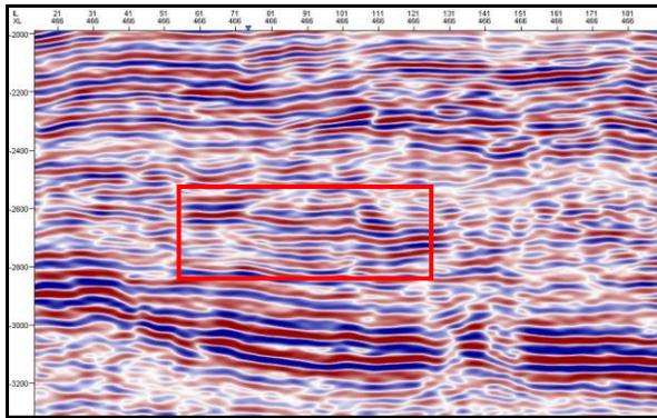
Figure 2(c): Median filter with filter width of 5X5 applied on original 3D PSTM seismic data. The highlighted part shows an increase in continuity and resolution of the event of interest
