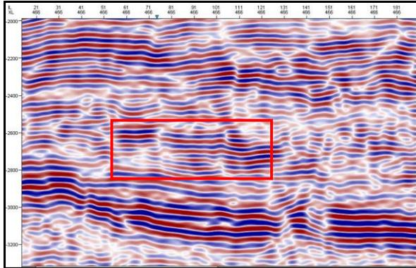
Figure 3(a): Graphic equalizer applied on the median filtered data to boost frequencies of interest. The highlighted area has better continuity of events which gives more confidence in seismic interpretation
