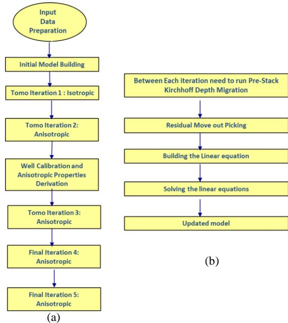
Figure 6: a) Workflow used for Velocity modelling (1 isotropic and 4 anisotropic) b) Tomographic velocity model building flow
