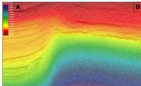
Figure 5: Final PSDM RMS Velocity model
