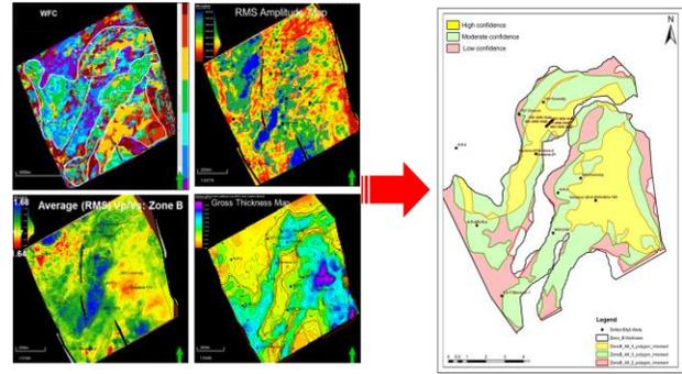
Fig-8 Deriving Sand Probability map combining all methods.
