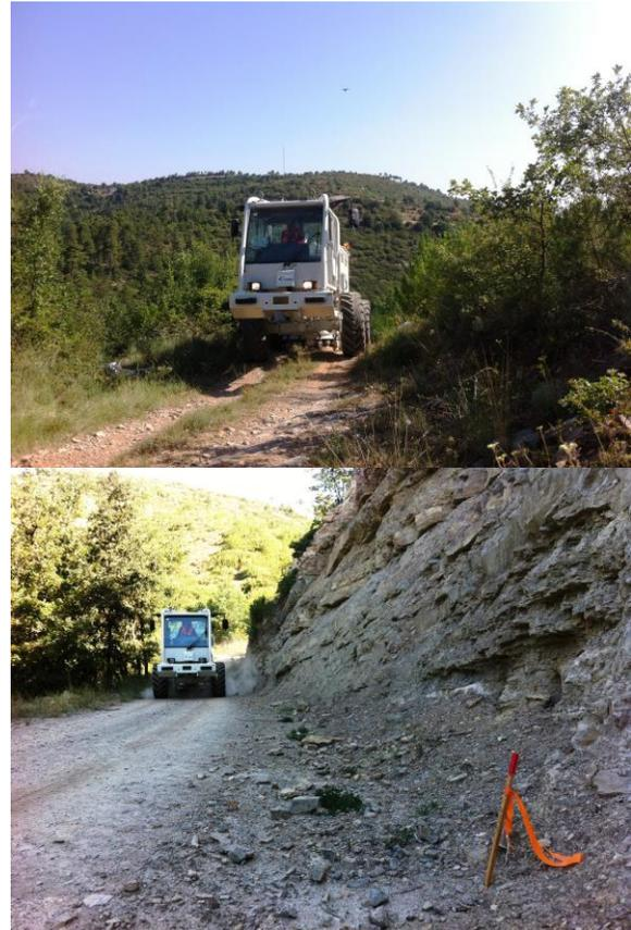
Figure 3: typical terrain conditions for potash mining in Spain, with the compact Nomad 15 vibrator in operation.
