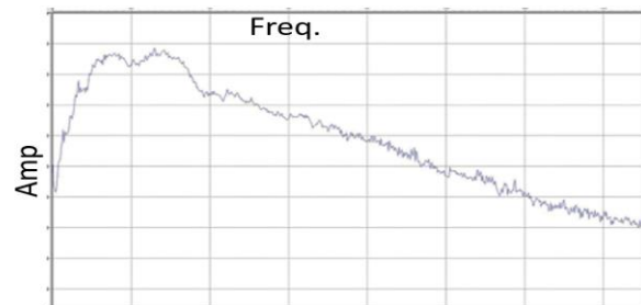
Figure 5: Amplitude spectrum for a single hole 20m, 5kg
