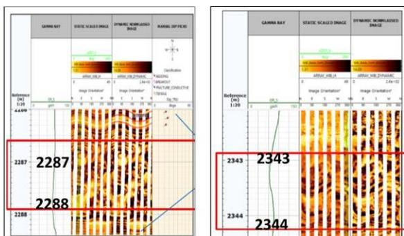
**Fig.5** Two different bedding directions observed. Possible thrust fault zone as marked by red box.
