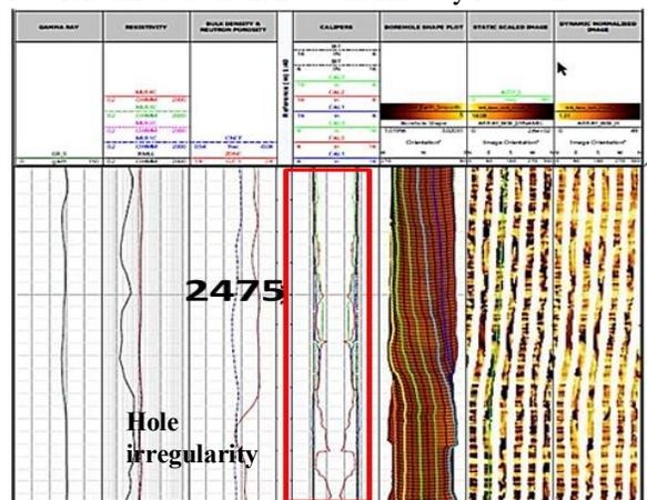
**Fig.6** Resistivity image log showing hole anisotropy due to severe break out in the interval 2466-2490m. Mud loss zone corresponds to the same interval
