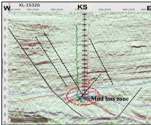
**Fig.8** Interpreted Crossline-15326 showing cross cutting of faults in well trajectory (*modified after KG Basin*)
