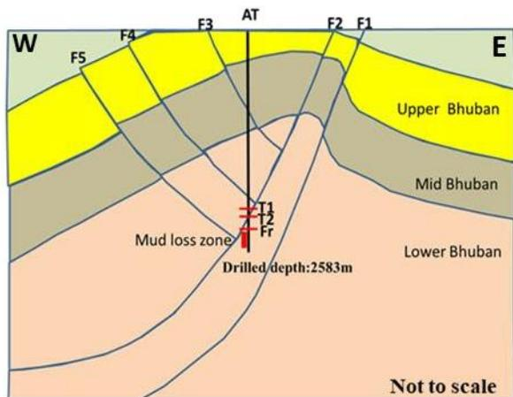
**Fig.4** Schematic geological section showing well AT and associated faults T1. Thrust-1 (2287m), T2: Thrust-2 (2345m) FR: Fractured/break out zone (2466- 2490m)
