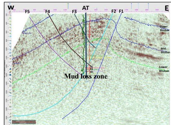
**Fig.3** Interpreted 2D section showing well AT; F1 indicates major thrust fault which was evident prior to drilling (After A & AA Basin).
