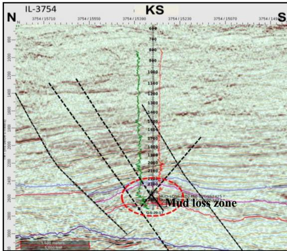
**Fig.7** Inline-3754 showing cross cutting of faults in well trajectory (*modified after KG Basin, unpublished ONGC work*)
