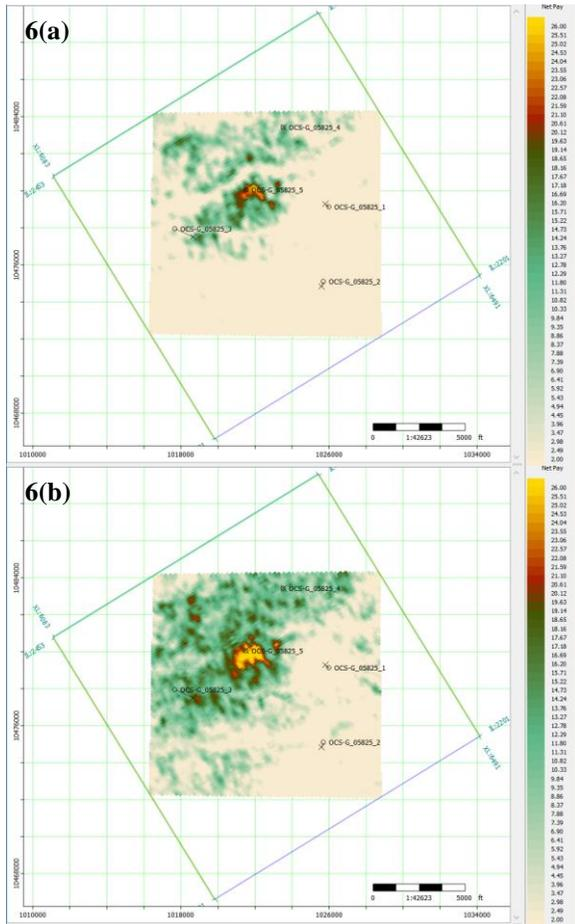
Figure 6: Hydrocarbon pore thickness estimation using PNN from a) conventional and b) direct workflow.
