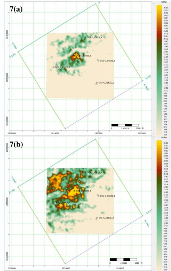
Figure 7: Hydrocarbon pore thickness estimation using DFNN from (a) conventional workflow and (b) direct workflow.
