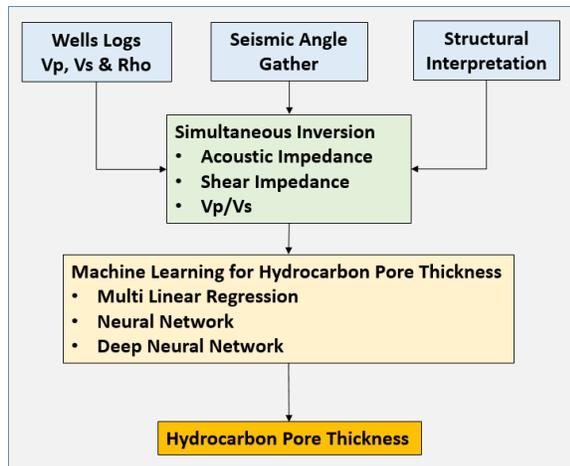
Figure 4: Workflow for direct hydrocarbon pore thickness estimation.
