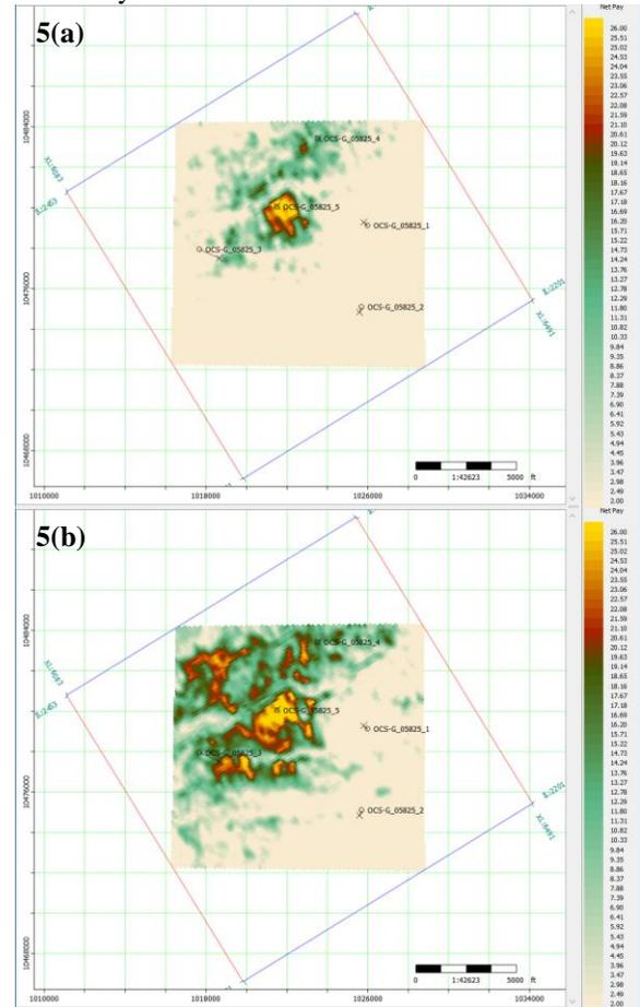
Figure 5(b): Hydrocarbon pore thickness estimation using multi linear regression from (a) conventional and (b) direct workflow.
