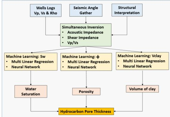
Figure 3: Workflow for hydrocarbon pore thickness estimation in a conventional way.
