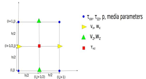
Figure 1: Staggered grid finite difference method for Poroelastic wave equation
