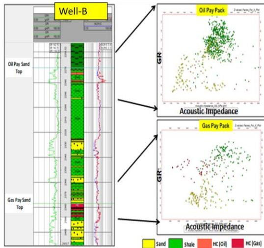
Fig. 7: Cross Plot between Gamma Vs Acoustic Impedance
