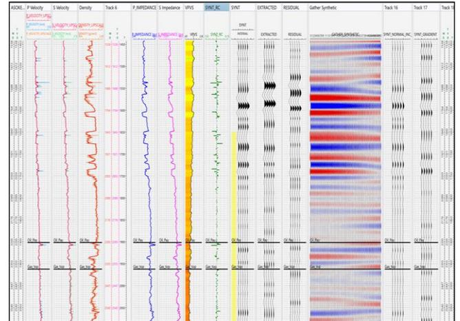
Fig. 6a: Synthetic Seismogram through well B
