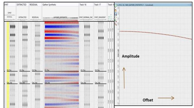
Fig. 6b: Amplitude Vs Offset along the gas-pay sand
