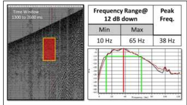
Fig. 13: Frequency Spectrum Analysis
