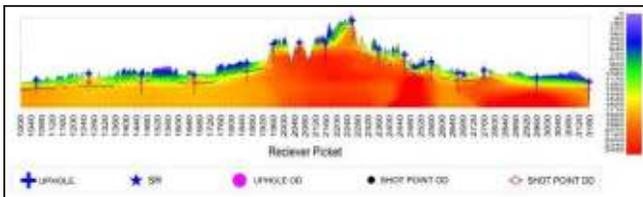
Fig.12: Near Surface Model of a seismic line across Atharamura Structure
