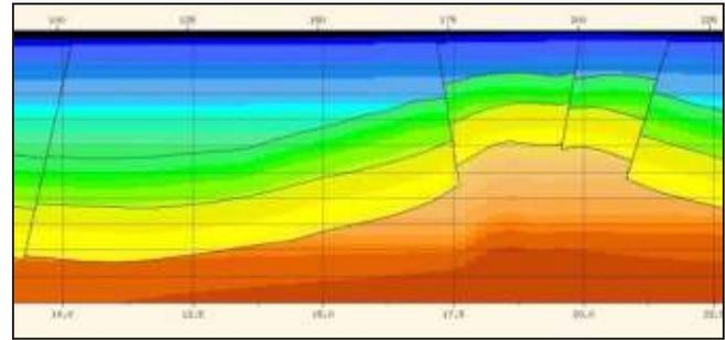
**Fig. 6:** 2D Model for a seismic line across Atharamura Structure
