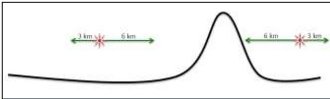
**Fig. 4:** Flip-flip up-dip ASS Shooting Pattern
