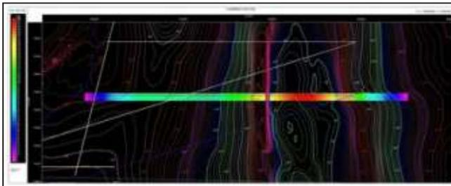
**Fig. 5:** Variable Fold Map with formation top contours
