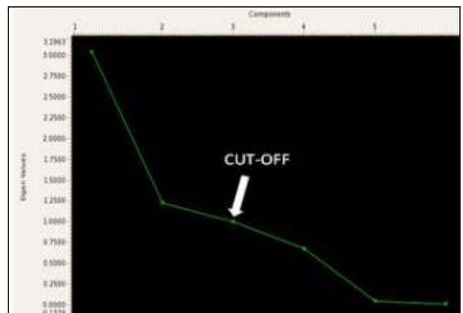
**Fig.5:** Selection of PC's with Eigen value cut-off  $\geq 1$ . PCs with value lower than 1 doesn't contain significant information.
