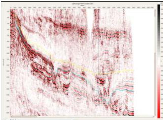
**Fig.3:** Seismic section and the interpreted horizons. The zone of interest for grid based facies analysis is within the two horizons. Dot represents a probable drilling location.
