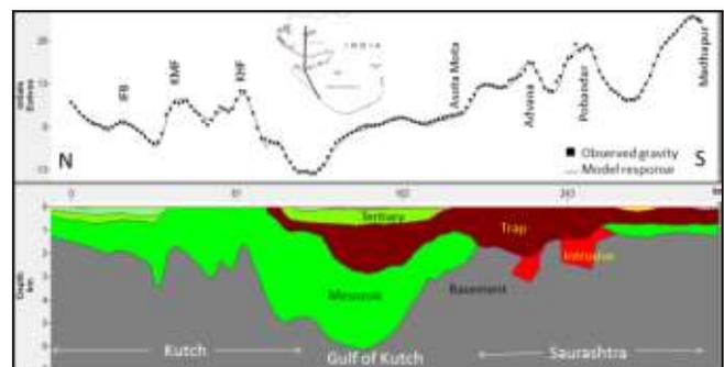
Fig. 6a: Gravity modelling of profile-1.
