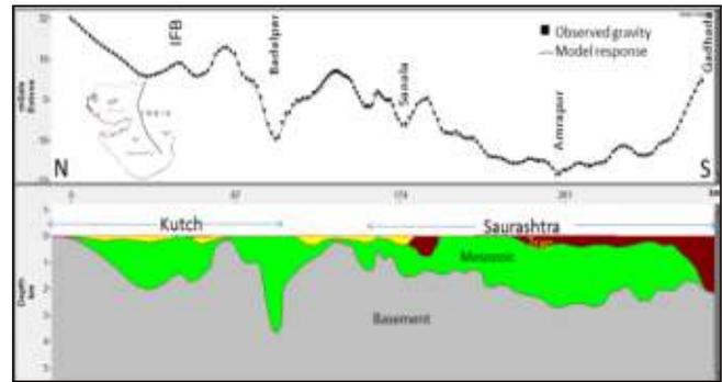
Fig. 8: Gravity modelling of profile-3.
