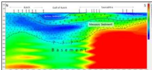
Fig. 5: 1D Occam-inversion section of profile-1.
