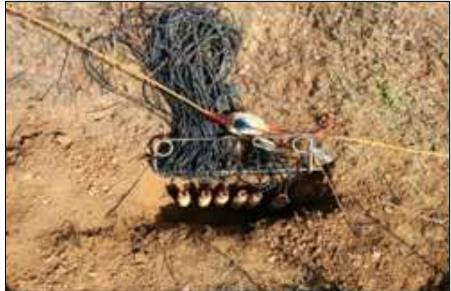
Fig. 5: Sensor Coupling in Pits
