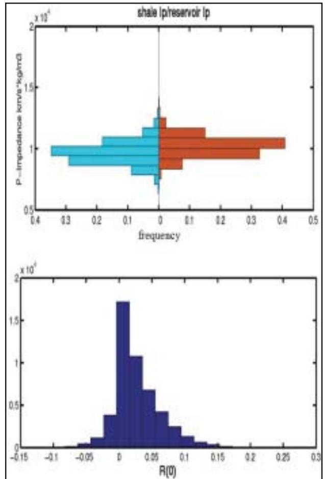
**Fig. 3:** a) Top: Distribution of shale and sand impedances used in the computation for Figure 2. On average the sand has slightly higher impedance than the shale, but there is considerable overlap. b) Bottom: Histogram of reflectivity from Monte Carlo simulations. Because of the overlap in shale and sand impedances, there is a small but finite chance of getting negative reflectivity values
