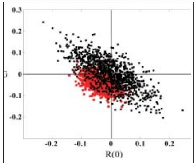
Fig.5: Monte-Carlo simulated synthetic  $R(0)$ - $G$  cross plot showing separation between two clusters; background in black and oil sands in red.
