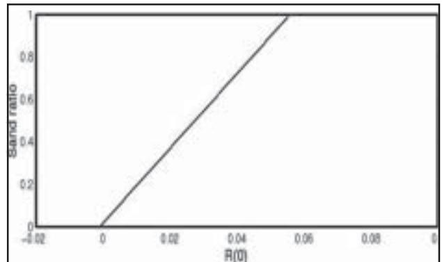
Fig. 1: Relation between normal-incidence reflectivity and sand/shale ratio in very thin-bedded sand-shale layers. The line is obtained using Backus average for thin layers, with blocked average values of sand and shale properties from well log. In this computation we ignored the variability of sand and shale velocity, density, and impedance.
