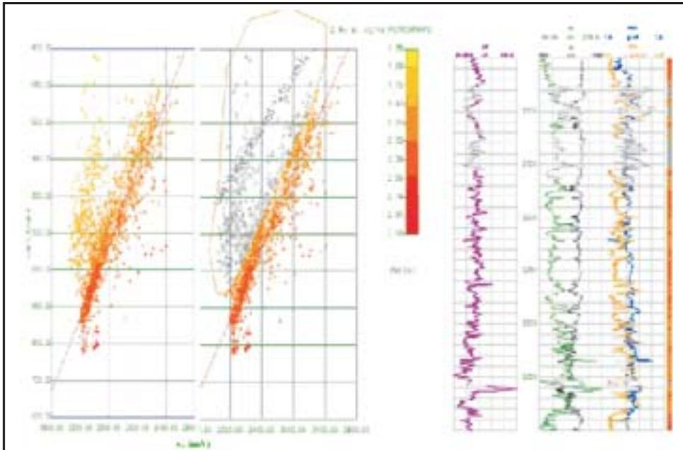
**Fig.3:** Vs plotted against vp shows the gross linear trend. Linear regression line fits the best after deselecting points corresponding to gas sands, oil and water sands. vp/vs is in colorbar axis. Deselected points are shown in grey color on log curve of corresponding interval. Well B.
