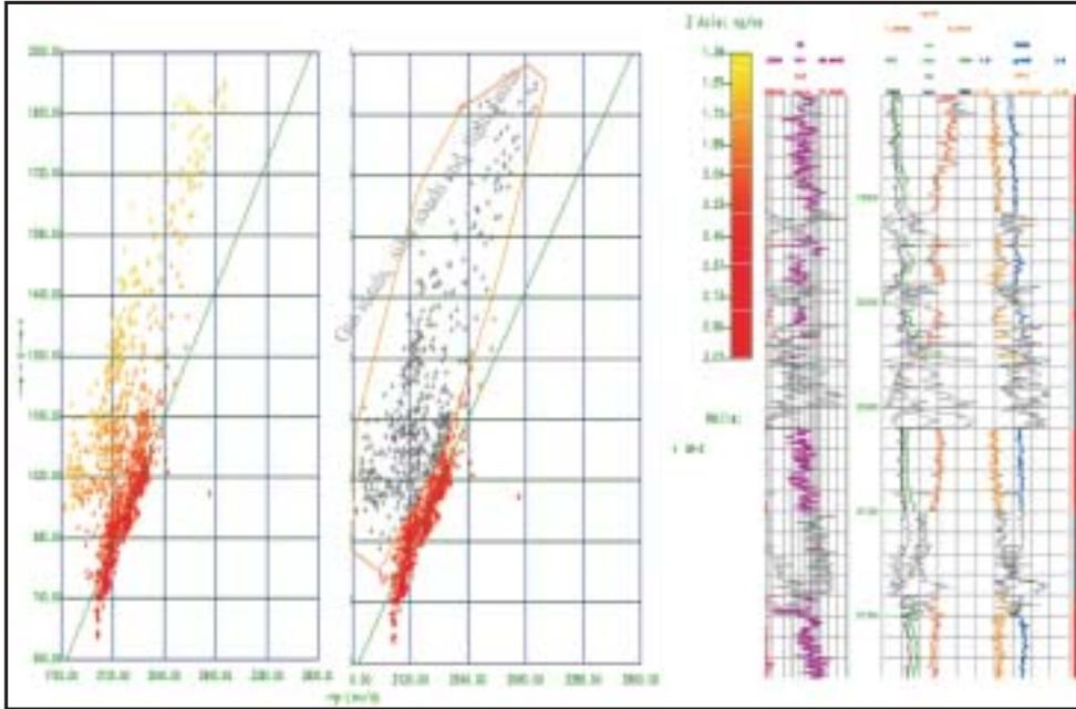
**Fig.2:** Mudrock line after deselecting points corresponding to porous and tight gas sands. Vp/Vs is in colorbar axis. Deselected points are shown in grey colour on log curve for corresponding interval; Well B
