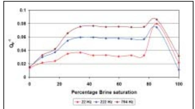
**Fig. 7:** ITF-51, Compressional attenuation with changing brine saturation. Differential pressure=6.89 MPa.
