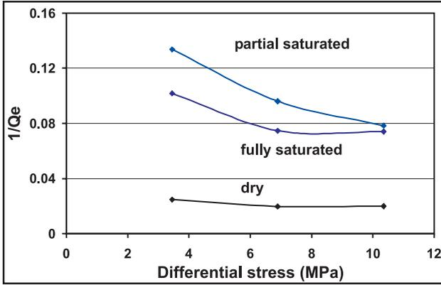
**Fig.3:** Rim sandstone, extensional (Young's)  $1/Q$  in dry, partially saturated and fully saturated rock with varying differential pressure (measurement frequency 1KHz). Porosity=0.19 and permeability=300 md .
