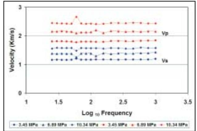
Fig. 2: Rim sandstone, compressional and shear velocity as a function of frequency and varying confining pressure. Porosity=0.19 and permeability=300 md.
