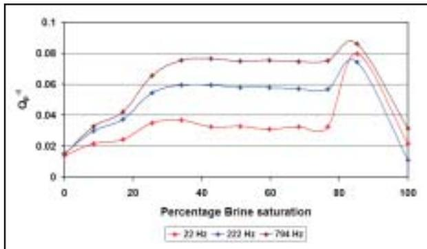
**Fig. 8 :** Uvalde carbonate, shift in attenuation peak with change in viscosity. The viscosity change is due to change in temperature of the heavy oil. Confining pressure=10.34 MPa. Permeability=550 md.
