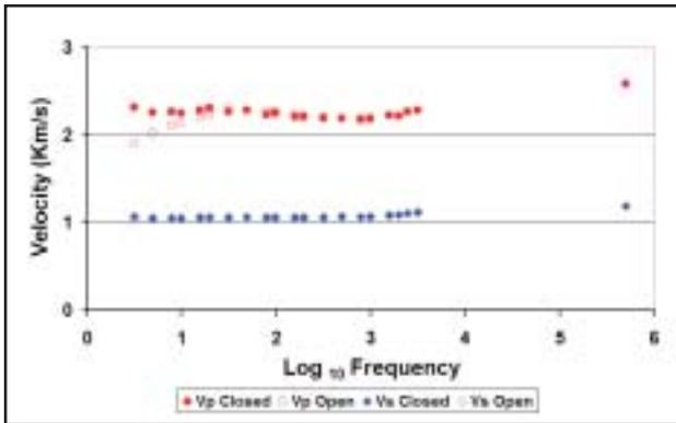
**Fig.5 :** Foxhill's sandstone, velocity vs frequency for open and closed boundary case. The sample is 100% saturated and the confining pressure is 17.3 MPa and the pore pressure is 6.9 MPa. Note the frequency at which both open and closed P-wave velocities become equal. Porosity=27% and permeability=100md.
