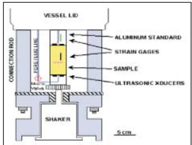
Fig. 1: Schematic diagram of the low-frequency apparatus.
