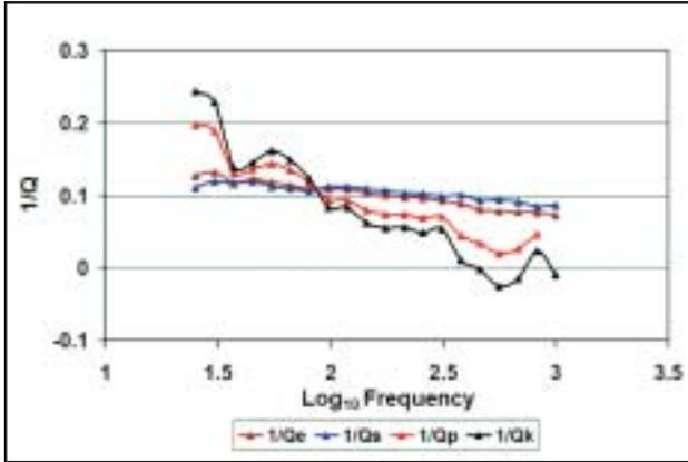
**Fig.4:** Rim sandstone, variation of extensional, shear, compressional and bulk 1/Q values with frequency at 100% saturation (open boundary). Note the reversal of order as we move from low to high frequency. Differential pressure=6.89 MPa.
