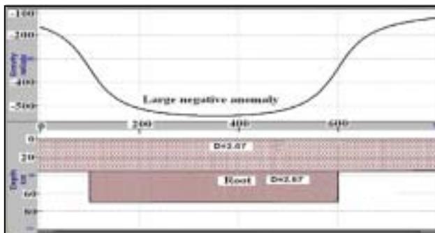
**Fig.3 :** Schematic model on gravity anomaly due to the root of the Himalayas.
