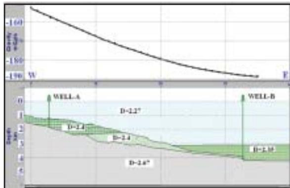
**Fig. 4b.:** 2D-forward gravity modeling along the profile AA' with sediments.
