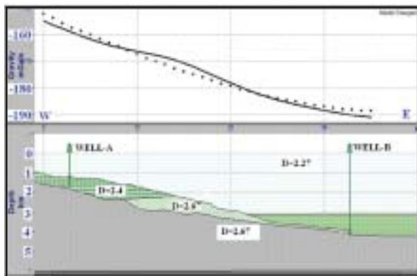
**Fig. 4a. :** 2D-forward gravity modeling along the profile AA' without adding sediments.
