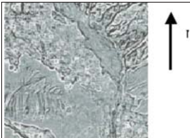
Fig.10 : Textural classified image of a part of Dun valley based on skewness (Window size: 7×7)
