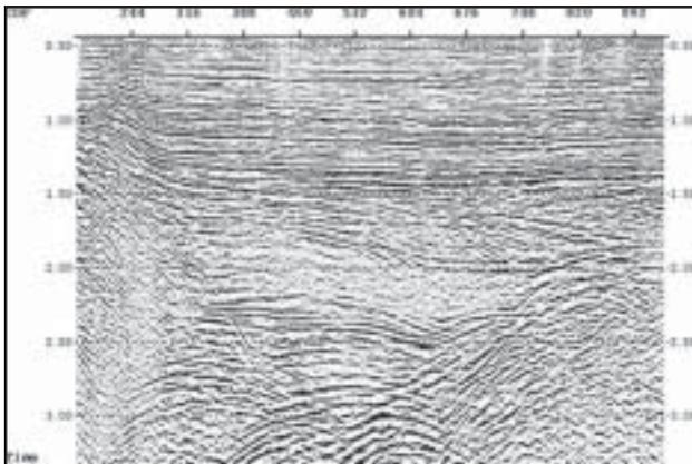
**Fig.2:** Linear dipping alignment of events
