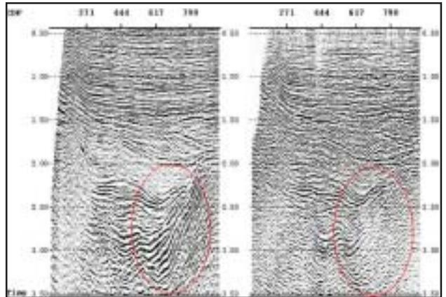
Fig.10: Comparison of PSTM stacks of unfiltered gathers (left) and filtered gathers (right).
