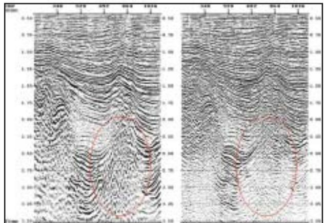
Fig.11: Comparison of PSTM stacks of unfiltered gathers (left) and filtered gathers (right) of other profile from the same area.
