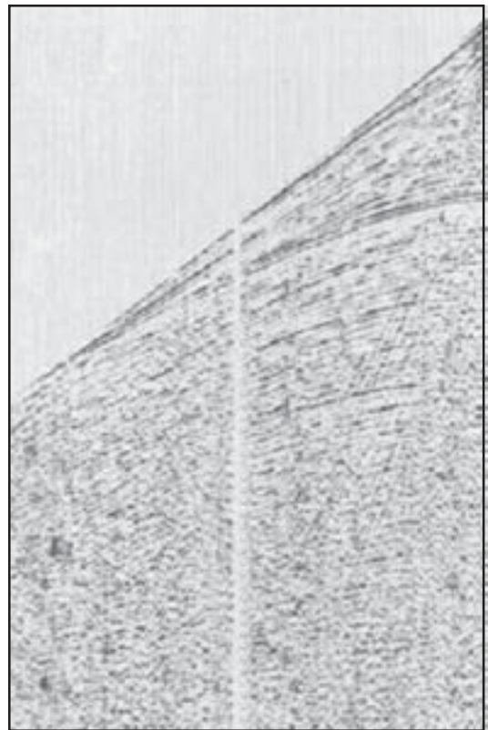
Fig.7b: Field monitor record at 35.5m in intermediate high velocity layer at uphole-3 location.
