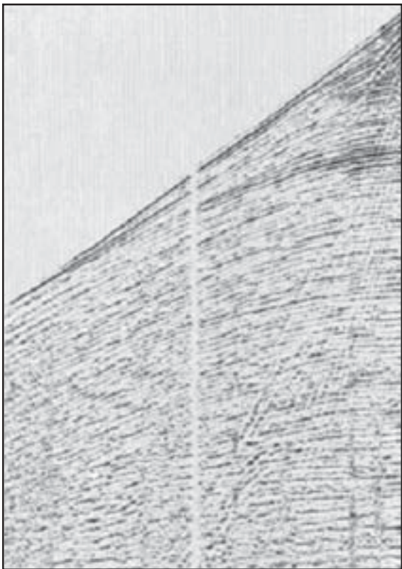
Fig. 7a: Field monitor record at 23.5m in shallow high velocity layer at uphole-3.
