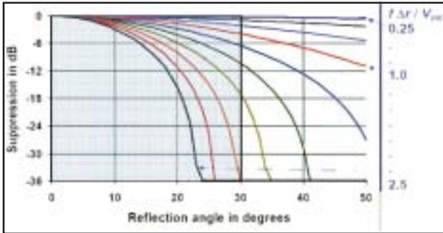
**Fig 3 :** From G. Vermeer - Effect of linear array on signal in 2D as function of reflection angle, frequency, array length and interval velocity. Many cable based systems force large spatial sample intervals causing high degrees of data suppression.
