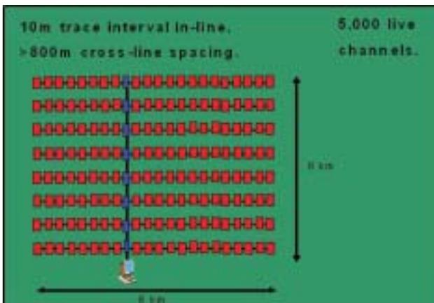
**Fig 4 :** The practical limit for cable-based telemetry systems? 5,000 live channels, 10m trace interval, >800m line spacing? The future for good data?
