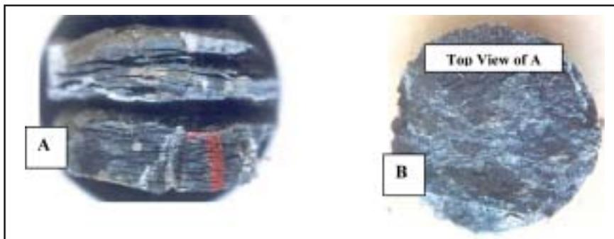
**Plate-2. Core Photographs of Well # B.** A Finely laminated carbonaceous shale/coal with siltstone interclations giving rise to splintery nature of the rock which may be responsible for development of reservoir facies. The visible splitting may be caused by dampness during storage at KDMIPE core house. The permeable paths are criss crossing each other. B. Top view of core also shows layering structure of coal/carbonaceous coal
