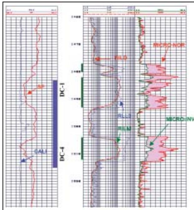
**Plate-4** Well # C Good gauged hole, Both coal units are permeable from SP & MEL logs. Resistivity moderate to high.
