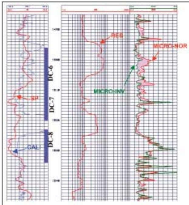
**Plate 3.** Well # B, X coal highly caved, Lower portion of X is More permeable on SP & Micro resistivity.
