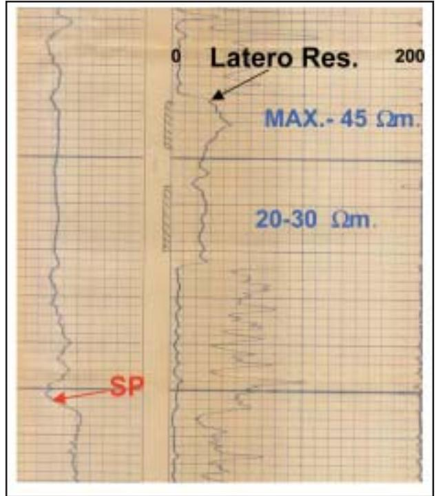
**Plate- 6.** Well # E, This well in the North western part of Kalol field Produced water @ 18 m<sup>3</sup>/D The resistivity is low and negative SP is developed in entire unit. The log responses and production data suggests that low resistivity coupled with SP indicates reservoir development.
