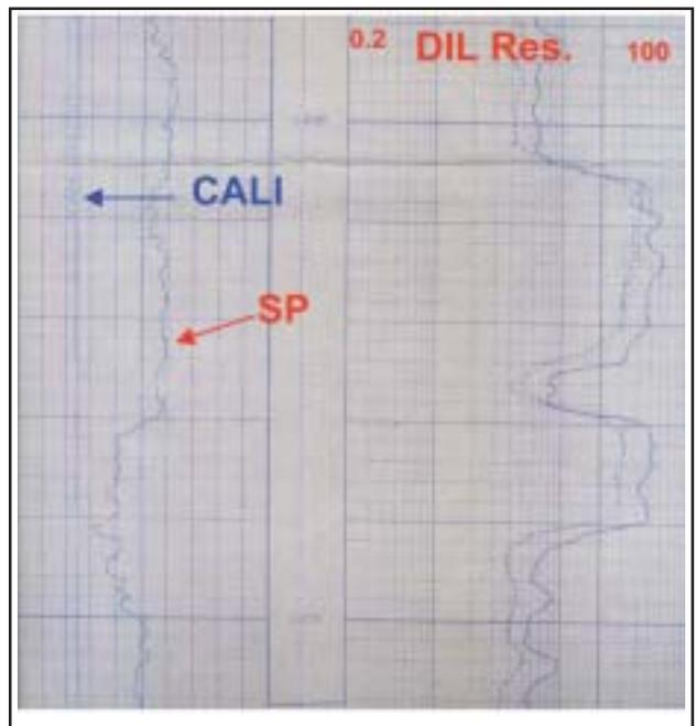
**Plate -7.** Well # F, Negative SP is developed in the interval 1465-75m. against X coal and underlying silt whereas no SP is seen against IX coal. This example Validates the response of SP exhibiting permeability character
