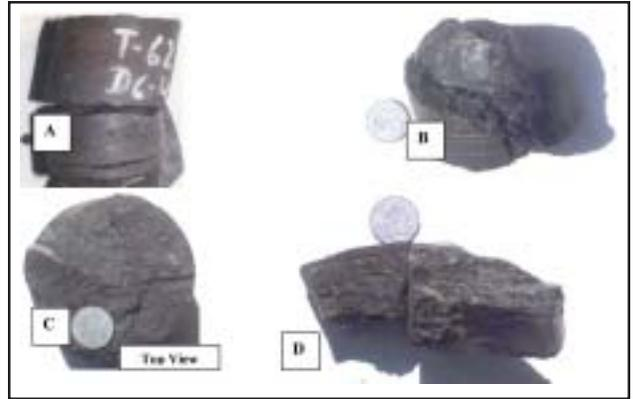
**Plate-1. Core Photographs of Well #A.** A. Carbonaceous coal showing permeability paths weak planes parallel to bedding planes., B. Coal showing conchoidal and sub-vertical fractures., C. Coal with vertical and sub-vertical fractures. D. Horizontal layering in coal.
