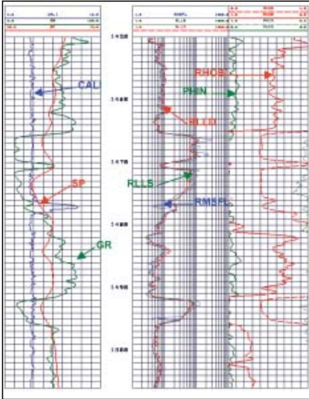
**Plate-5** Well # D, Southern part of main block, Gradation from coal to shale via carbonaceous shale from 1474 to 82 m, evident from resistivity, GR and density logs. Good development of SP against laminated carbonaceous shale also. Gradation also observable in X coal.
