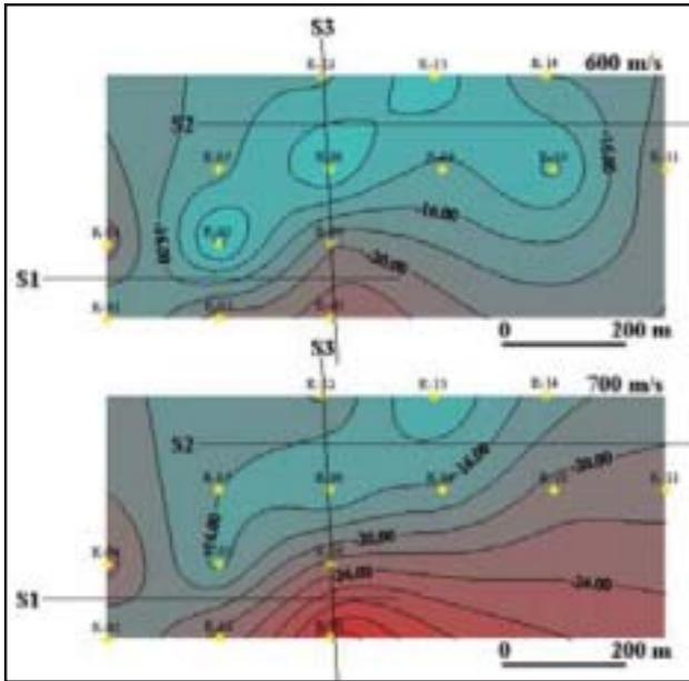
**Fig. 4 :** Engineering seismology case study: The S-wave velocity-depth contours over the site. The contours correspond to the maximum depths associated with 600 m/s (top) and 700 m/s (bottom) S-wave velocities.
