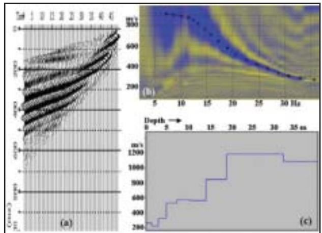
Fig. 3 : Engineering seismology case study: (a) Surface waves in a field record from a refraction profile (K09) after inside and outside mute to remove refracted and reflected waves; (b) the dispersion curve for the Rayleigh fundamental mode interpreted from the phase velocity spectrum; (c) the S-wave velocity-depth profile estimated from the inversion of the dispersion curve.
