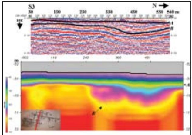
Fig. 2 : Engineering seismology case study: The seismic section (top) derived from the analysis of reflected waves and the P-wave velocity-depth model (bottom) derived from the analysis of refracted waves. Horizon A defines the boundary between the top soil and the lake deposits, whereas horizon B defines the boundary between the soil-bedrock interface.
