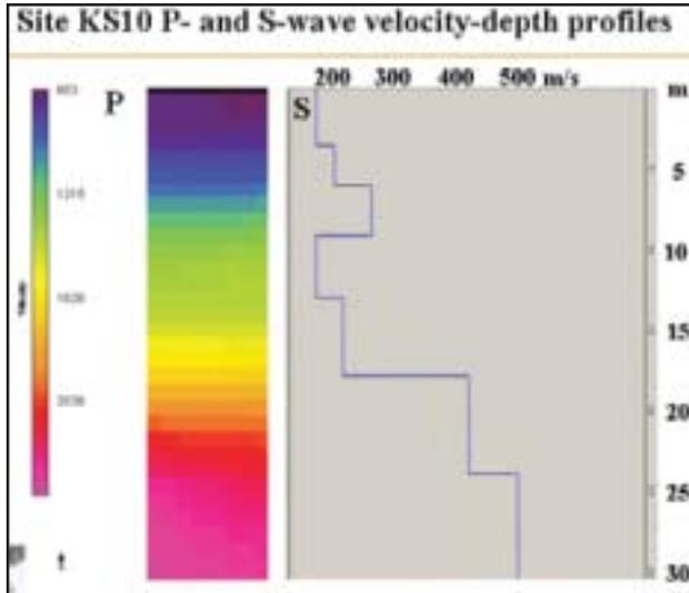
**Fig. 1** : Earthquake seismology case study: The P-wave velocity-depth (left) and the S-wave velocity-depth (right) profiles down to 30-m depth.
