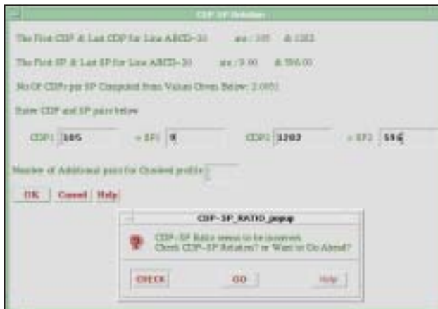
Fig.3. Dialog box for entering acquisition parameters. Entry is done once for the first line in each investigation. The values entered are stored and prompted and alteration, if any, only need to be done for subsequent lines
