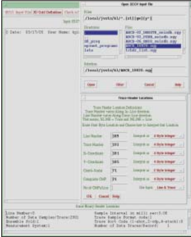
Fig. 8. The main window for EpinetSgycpy3d. Insets show the segy file selection dialog and trace header location definition dialog.
