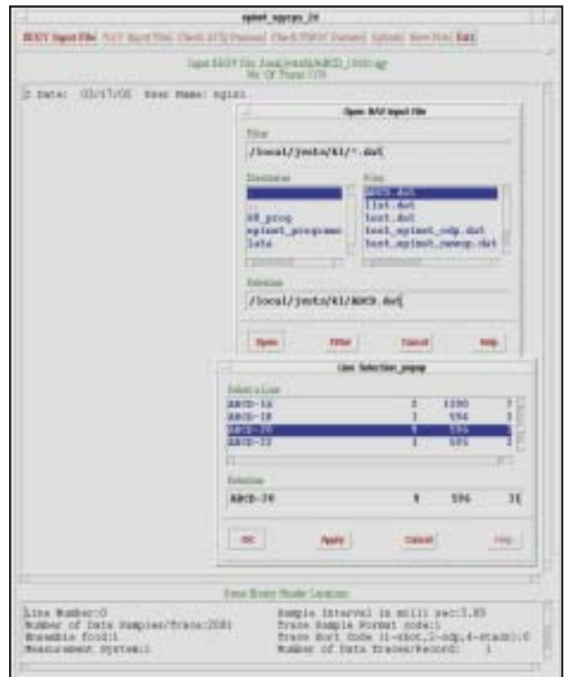
Fig.1. The main menu of ‘EpinetSgycpy2D’. The insets displayed are popup menus for selecting the navigation input file and the seismic line from the list of lines within the navigation file selected.
