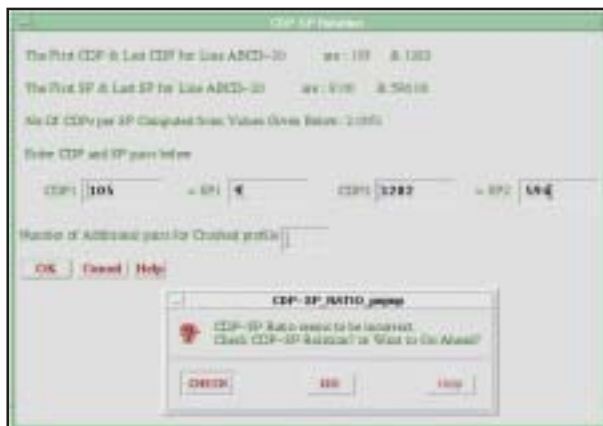
Fig. 2. Dialog showing the available range of CDP values from seismic and available SP values from navigation data. The inset shows that directly relating the CDP range with SP range is incorrect. User needs to provide correct relation considering the spread geometry with respect to shot point.
