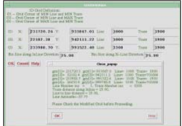
Fig.9. 3D grid definition. The inset shows the four computed grid corners, line and trace number increments and azimuth for QC check.
