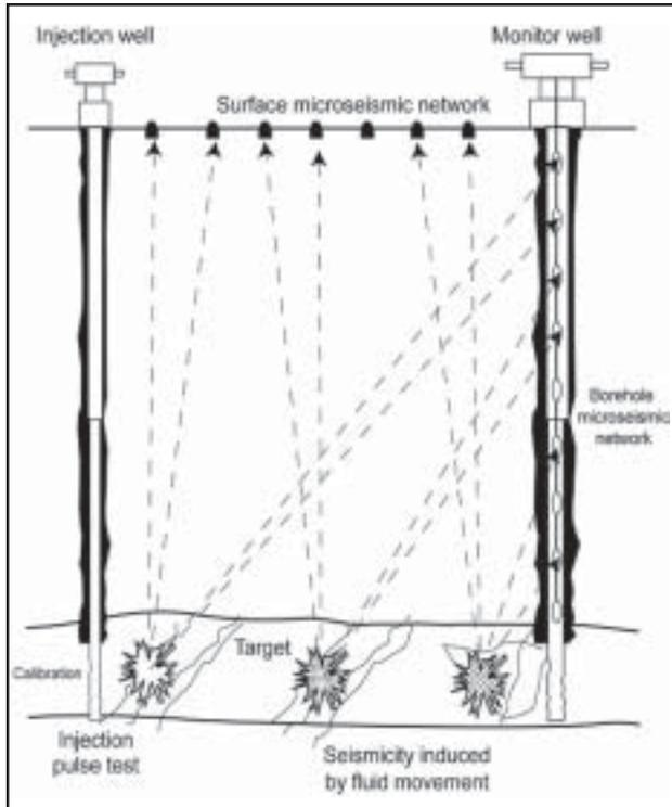
**Fig. 2** A network of 3-component sensors permanently cemented in boreholes and on ground surface measure events triggered in the reservoir. Microseisms or minute earthquakes are induced by reservoir rock slippage with reservoir fluid movement.
