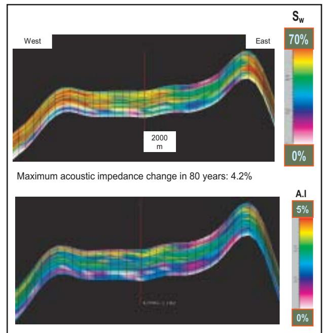
**Fig. 3.** Water saturation ( $S_w$ ) changes from the fluid simulation model for year 1953 to 2032 and the resultant acoustic impedance (AI) change over the same time period
