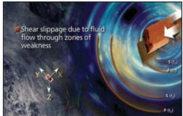
**Fig.1.** Reservoir production and injection operations create stress perturbations induced by shear stress release and cause shear slippage along zones of weakness in reservoir rocks. Minute earthquakes emanated along the elastic failure surface are recorded in 3-component seismic sensors.
