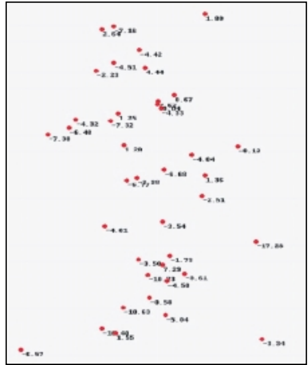
Figure 6: Showing mis tie map corresponding to Reflector C after map migration using 3D velocity depth Model (including vertical gradient and anisotropy)
