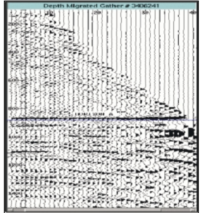
Figure 3: An APSDM Gather. Note the flatness of event at farthest offsets (depth/offset ratio \approx 2.4) 5Km N
