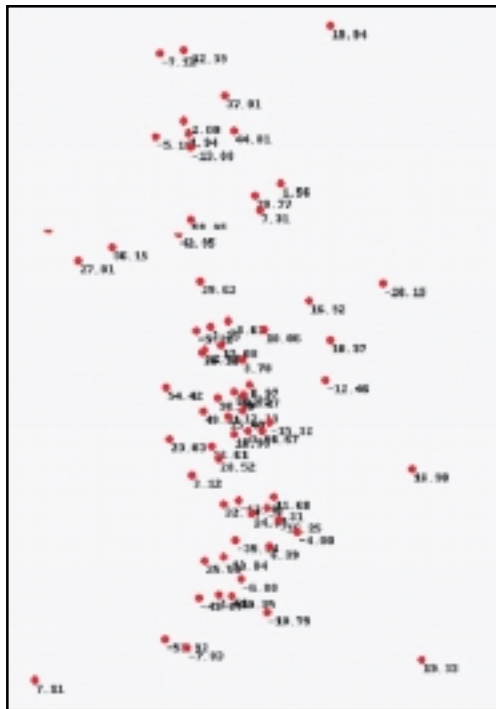
Figure5: Showing mis tie map corresponding to Reflector A after map migration using 3D velocity depth Model (including vertical gradient and anisotropy)
