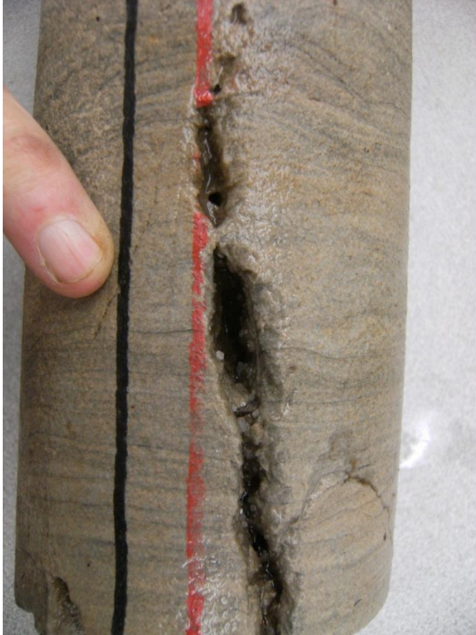
Figure 4: Dissolution along a fracture plane in the Arbuckle dolomite of Kansas created highly irregular fracture widths that were later partially filled with calcite mineralization.
