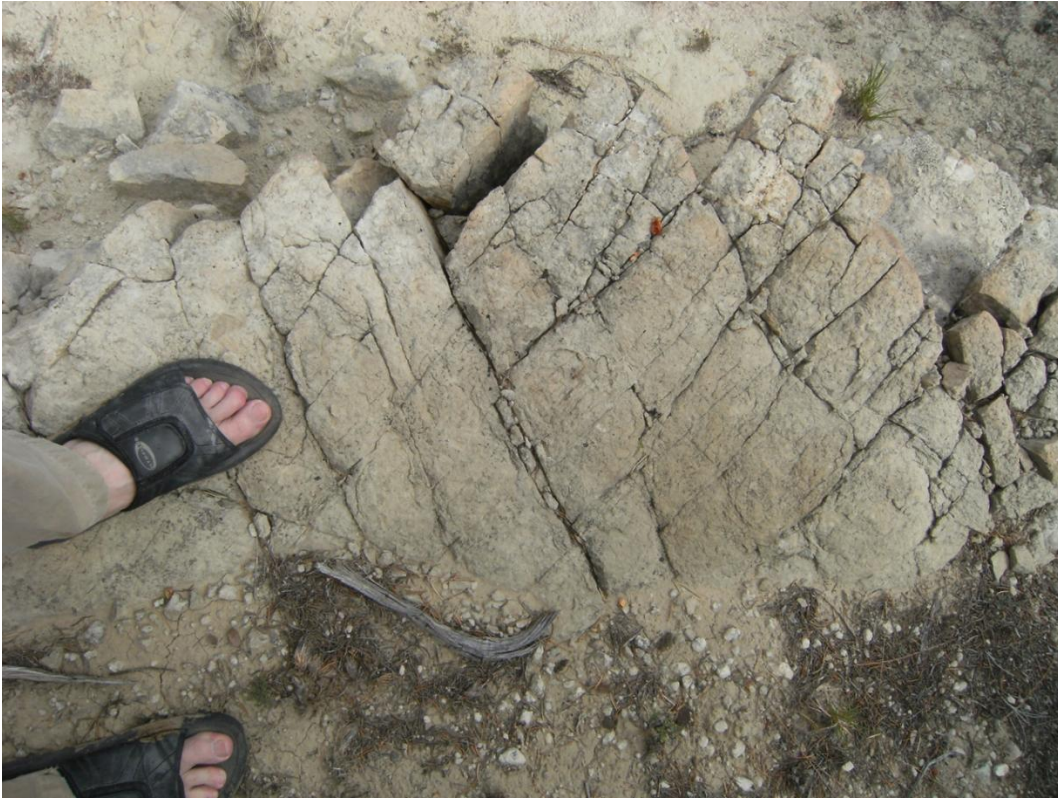
Figure 7: A set of vertical, bed-normal, right- and left-lateral strike-slip conjugate fractures, formed in a stress regime where the maximum compressive stress was in the horizontal plane, bisecting the acute conjugate angle, i.e., from top to bottom of the photograph. We are looking at a silty zone within the Mancos Shale in New Mexico. Shear fractures may also form as low-angle reverse-dip-slip conjugate pairs.
