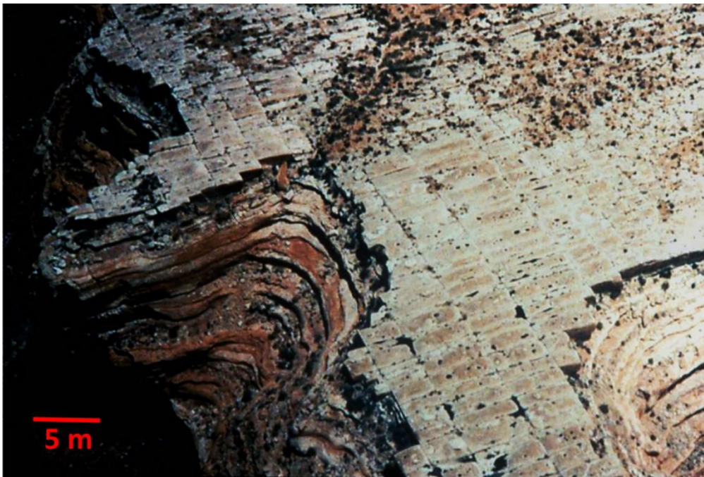
Figure 2: Aerial photograph of superimposed sets of extension fractures, which could create relatively isotropic horizontal permeability provided they have similar widths and degrees of occlusion by mineralization. This example shows Cedar Mesa Sandstone from Utah.
