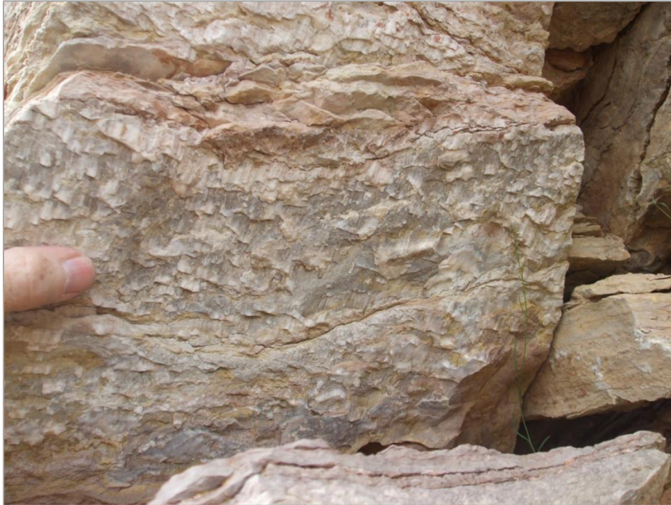
Figure 8: The face of a shear fracture displaying lineations and stepped mineralization indicating oblique shear and offset both before and after mineralization. This example shows Madera Limestone from New Mexico.
