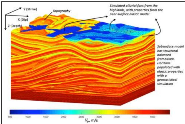
**Fig. 5:** Perspective view of the digital Foothills model. 3D rendering of the grid of compressional wave velocity
