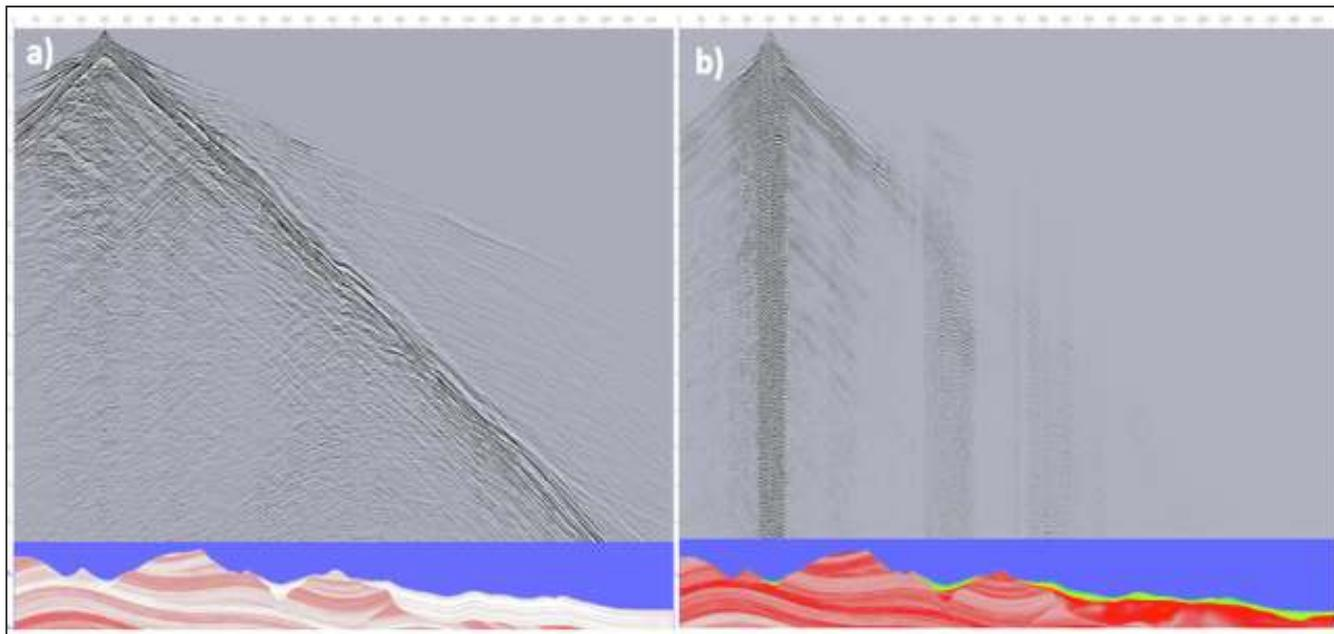
**Fig.** a) Synthetic shot using initial near velocity model, velocity defined by conformed layers. b) Synthetic shot from improved near velocity model including lateral variation in alluvial fan showing more scattering of surface waves and reverberation between near and subsurface features.
