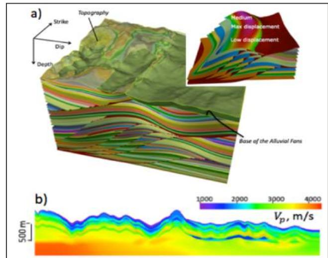
**Fig. 2:** Structural framework of the Foothills model. a) Displacement variation along strike for the deeper structures. b) Starting near velocity Foothills model.
