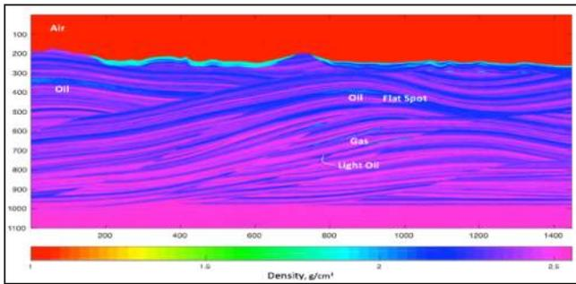
**Fig. 4:** Hydrocarbons. Density cross section. Elastic properties and density set to values of sediments with hydrocarbon charge. The color scale is clipped at the low end to 1.
