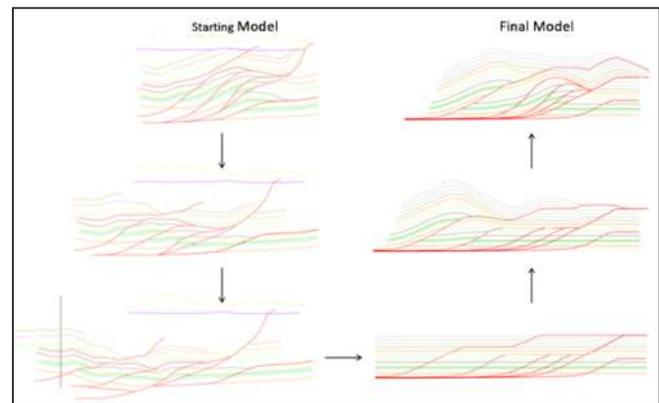
**Fig. 3:** Building the structural framework. Restoration and redeformation.
