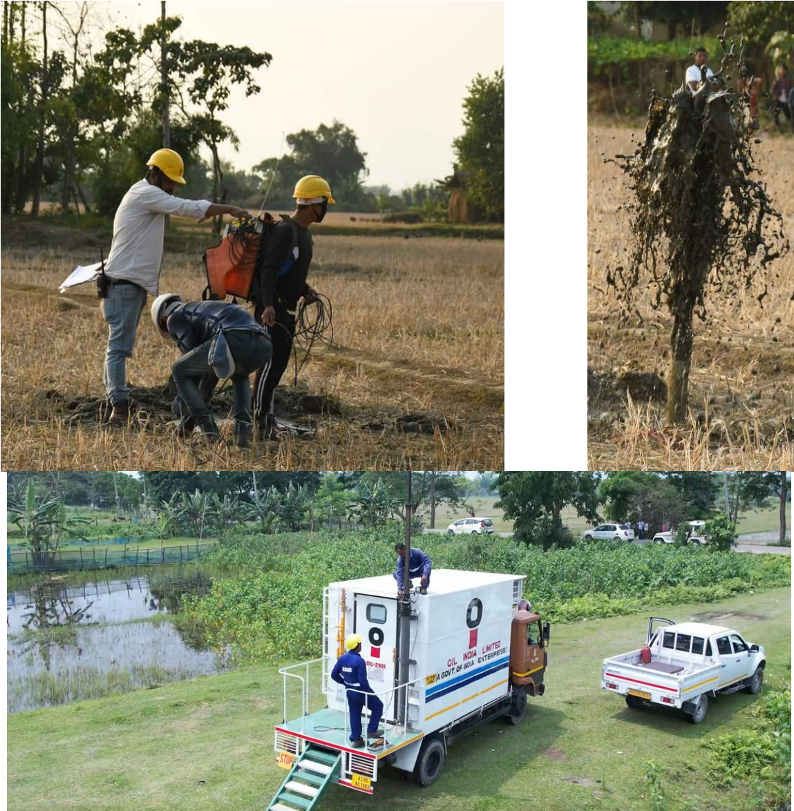
(Seismic survey in Assam. Top Left: Preparing for the shot. Top Right: A shot being taken using an explosive source. Bottom: Truck with wireless recording capabilities.)
