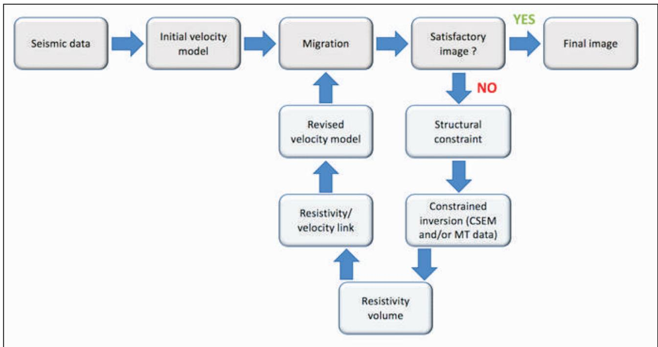
**Figure 4:** Workflow applied in the example presented here. The top row, shaded grey, represents a standard seismic imaging workflow. Adding the multi-physics loops, shaded blue, can dramatically improve the seismic image that is obtained.
