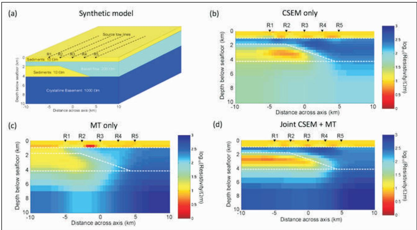
**Figure 2:** Simple 2D synthetic example illustrating the benefit of combining CSEM and MT data. (a) Synthetic model representing a basalt flow, sub-basalt sediments and basement. Synthetic CSEM and MT data were generated from this model, assuming five seafloor receivers (R1-R5) and five along strike source tows. (b) Inversion of the CSEM data alone. (c) Inversion of MT data alone. (d) Joint inversion of the CSEM and MT data. See text for discussion.
