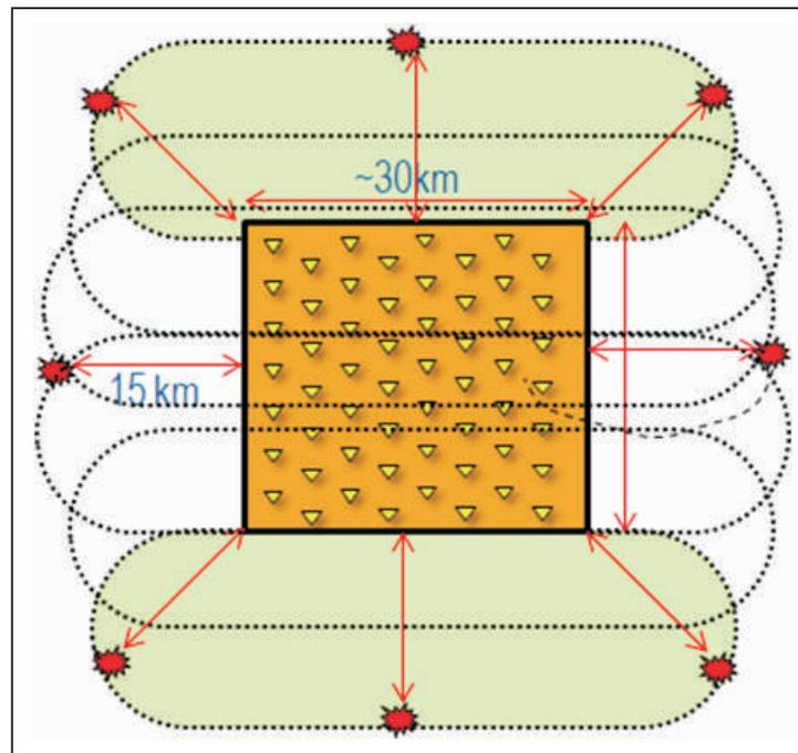
**Figure 5:** Areal layout of nodes (triangles) and source/streamer lines (red stars on dashed lines).
