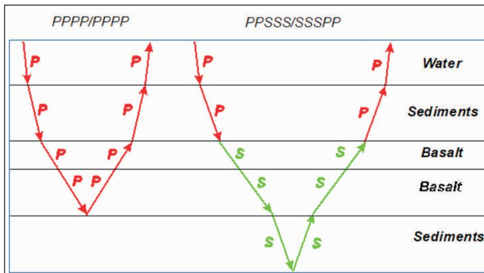
Figure 1: Simple 2D model showing P and converted mode propagation paths through basalt.
