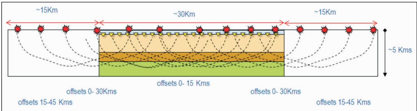
**Figure 4:** Ultra long offset acquisition model through basalt layer (dark orange) showing diving rays (dashed lines).
