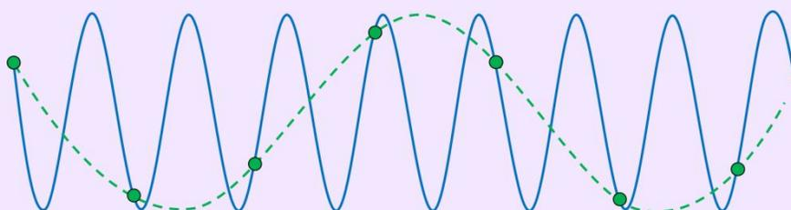
Figure 1: Sampling of a sinusoidal signal at greater than half its time-period and the resulting low-frequency dashed aliased waveform.
