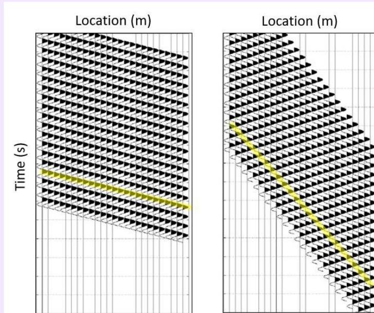
Figure 2. Aliasing in two dimensions. Both images show a suite of reflectors dipping to the right along the yellow trend. However, the human mind and computer processing algorithms will “see” the left-dipping alias in the image on the right image. In contrast, they will not “see” the steeply left-dipping alias on the left image. (After Hatton et al., 1986).
