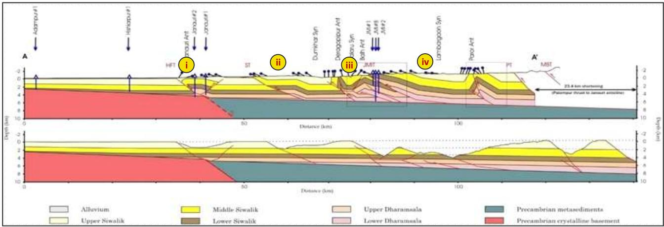
Fig. 3a: Preparation of Balanced cross section in Jawalamukhi area by Powers, Lillie and Yeats (1998)
