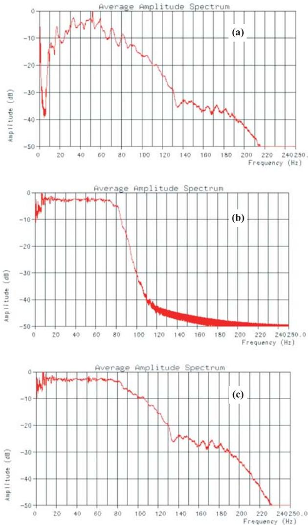
Fig. 9. The spectra of (a) the raw input (b) deconvolved data (with zero phase b.p. filter) and (c) with minimum phase b. p. filter.
