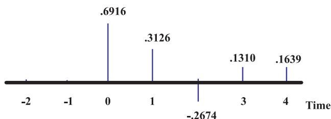
Fig. 1(b). Result of applying a 3-point spiking deconvolution on the input Fig 1(a) with Least Square Error=0.308364
