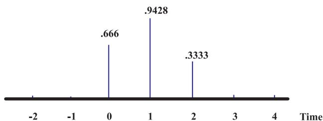
Fig.1(a). A minimum phase wavelet corresponding to equations (43) and (47).
