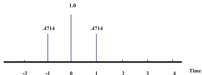
Fig. 2(a). A zero-phase wavelet corresponding to equations (35) and (53). By design, this wavelet and the minimum phase wavelet in Fig 1(a) have the same spectrum given by equations (44) and (48).
