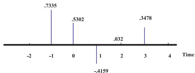
Fig. 2(b). Result of applying a 3-point spiking deconvolution on the input Fig 2(a), with Least Square Error=1.0537.
