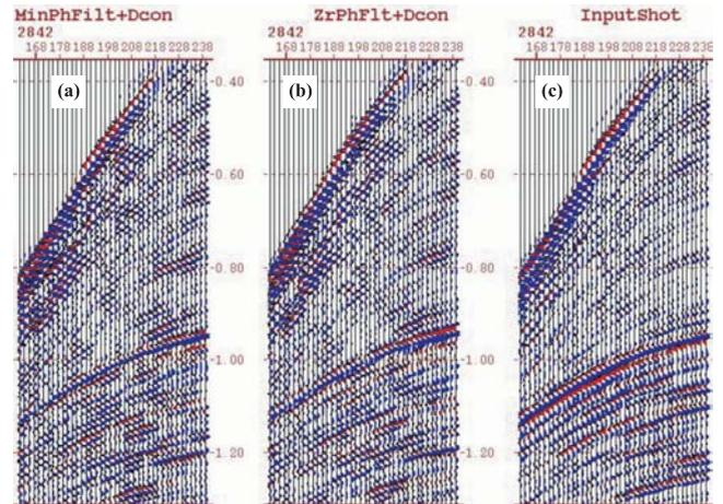
**Fig. 8.** (a) Result of applying minimum phase filter followed by a spiking filter. (b) Result of applying zero-phase filter followed by a spiking filter. (c) The raw data used for input for the processes in figures (a) & (b). Observe the higher resolution (and better stand-out) of events for the minimum phase pre-decon filter (a) as compared to that for the zero-phase case (b).
