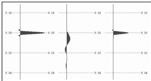
Fig. 4. An input with a spike at 200ms with a random noise of 0.01%. (b) The result of applying a minimum-phase band-pass filter. (c) Result of applying a one-sided spiking deconvolution to the filtered wavelet in (b). Compare the results with those in Fig. 3.
