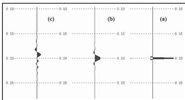
Fig. 3. An input with a spike (extreme right) at 200ms with random noise of 0.01% (b) The result (middle) of applying a zero-phase band-pass filter (c) Result of applying a one-sided spiking deconvolution to the filtered wavelet in (b). Compare the results with those in Fig. 4
