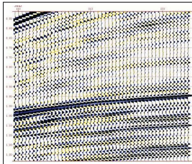
Fig. 5. The effect of zero-phase filtering a sample marine record with filter parameters (4 Hz, 12 db/oct, 60 Hz, 72 db/oct). The filtered output is shown in blue, while the input is shown in yellow. Black indicates the overlap between the input and the filtered output. Apart from the side-lobes associated with zero-phase b. p. filters, the positions of the peaks and troughs of the input are not altered.
