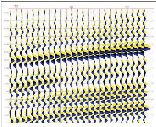
**Fig. 7.** Comparison between the minimum phase filtered output (in blue) and the zero-phase filtered output (in yellow). Note the time-shift of the former.
