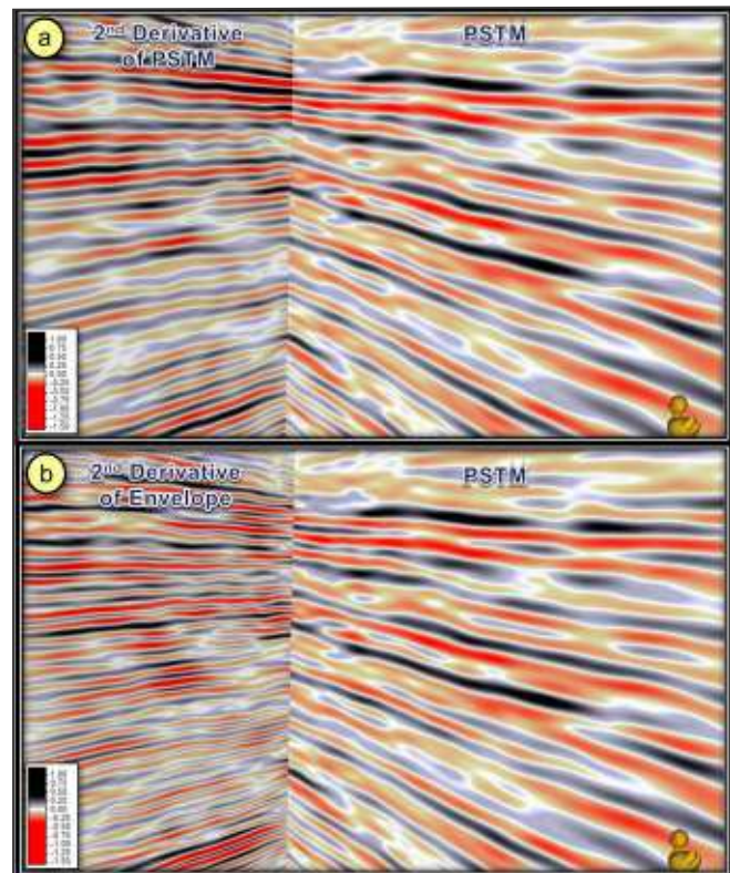
Fig. 6: (a) A 3D perspective view comprising the PSTM seismic inline to the right, and a crossline from the second derivative of PSTM data, which shows an incremental enhancement in frequency. Fig. 6(b) The same 3D perspective view but with equivalent second derivative on envelope attribute data shown to the left. This display enhances the reflection detail and hence the interpretation of subtle events and geobody geometries.
