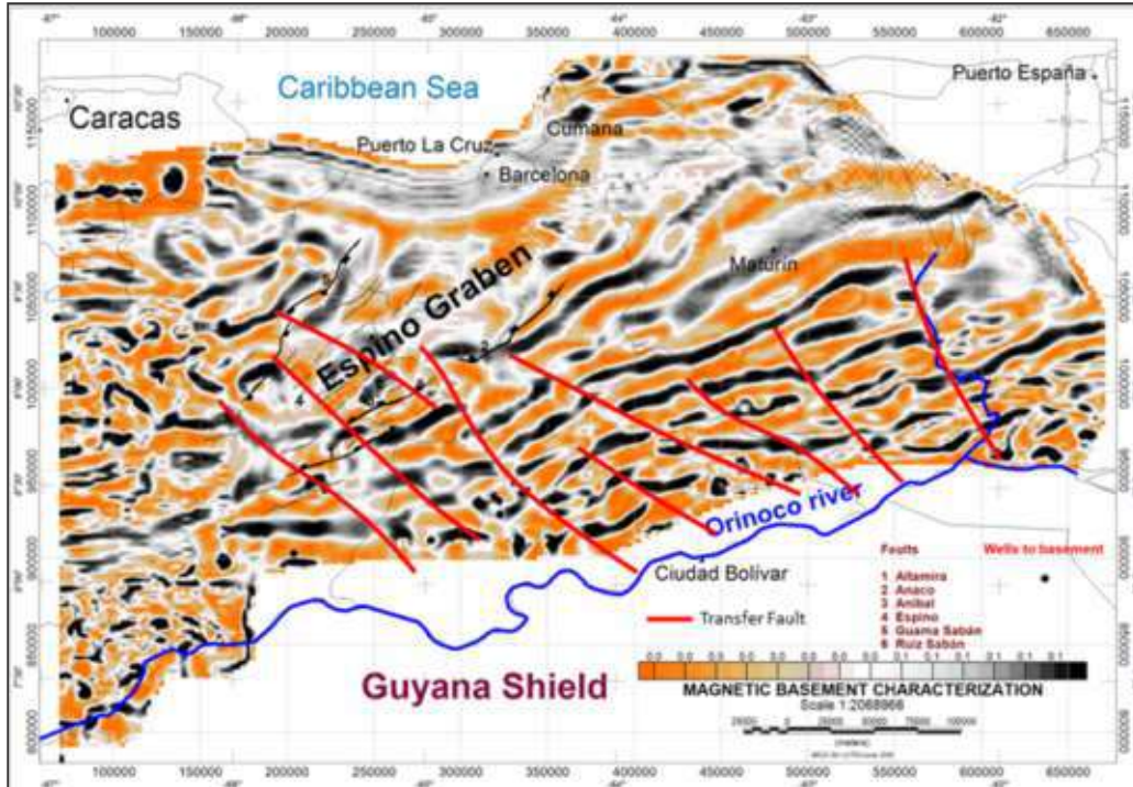
Fig. 8: Espino Graben magnetic basement characterization: the transfer faults due those changes orthogonal to oblique extension.
