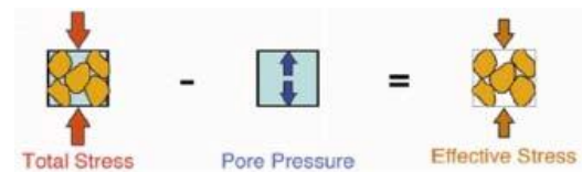
Fig.1 Showing the relationship between overburden pressure and the pore pressure i.e. Terzaghi's principle. (Terzaghi, 1943)
