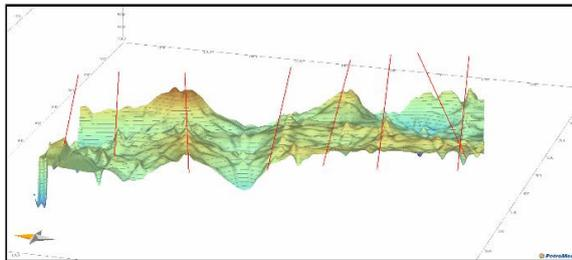
Fig. 7: Depth map of regional 3D model after interpolation and smoothing process (view to the East). This image shows clearly, that the structures are positioned along the seismic lines in red.
