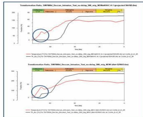
Fig 8: Time curves showing red curves for temperature and black curves for transformation ratio in two pseudo-wells. The kink in the black line (transformation ratio) shows the effect of the first intrusion event.
