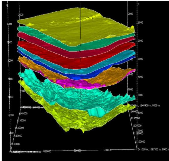
Fig. 6: 3D View of depth maps around deepwater well in PetroMod SeisStrat 3D
