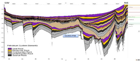
Fig. 5: Line GXT-1 illustration of the petroleum system elements (PSE) assigned to the 2D models. Note that the two lower layers within the Cochin Formation are considered as underburden.
